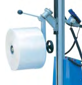
Attachment A-4 is a roll handling attachment designed to handle rolls in the vertical and horizontal position (poker chip position). The unit features an expandable ram that hold the roll by expanding in the core and turning the wheel pictured. The ram is 11" long and is 2.9" in diameter.
