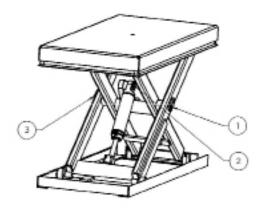
1-Central Pivot2-Cylinder Coupling Pin (Elevated Cycles)3-Central Pivot
