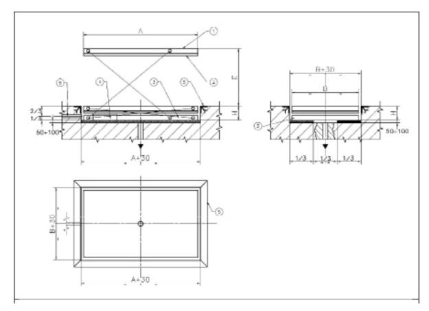
Hole length = A+30Hole width = B+30Hole depth = height of the closed table (Attention, some options may change the dimension of the pit)
